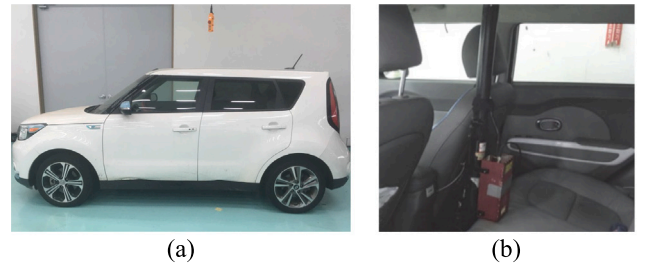
Fig. 11. Experimental set-up. (a) Test vehicle; (b) RT-3002 for verification.
