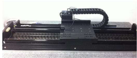
Fig. 10. Experimental prototype PMLSM system.
