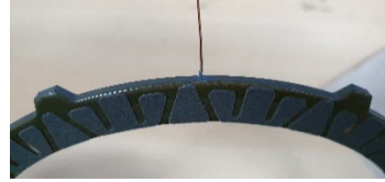
Photo. 3 Installation of the thermistor in the clutch plate.
