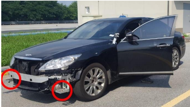
Figure 1. An ultrasonic look-ahead sensor module under the front of the vehicle for vehicle predictive control.
