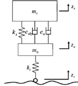
Figure 1. Quarter-car model of the semi-active suspension system.
