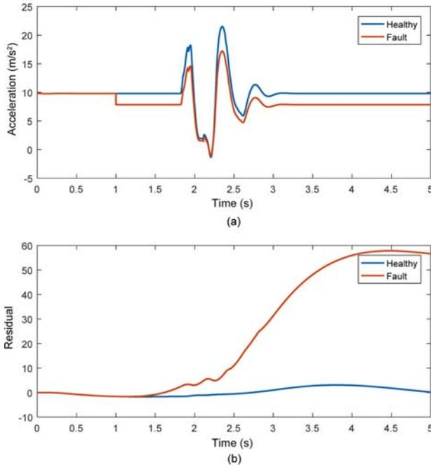
Figure 8. Speed-bump simulation results for residual generation (gain fault): (a) Front left sprung mass acceleration; (b) Residual generated by the unknown input residual generator.
