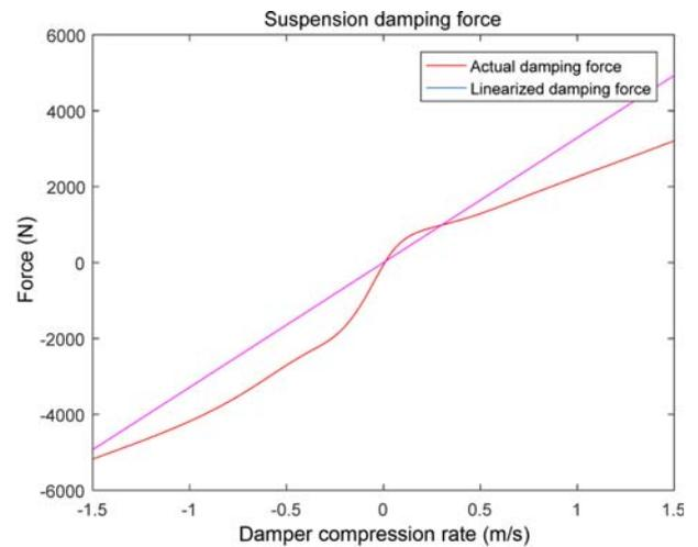
Figure 2. Linear and nonlinear damping characteristics.
