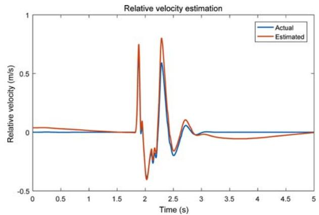
Figure 10. Speed-bump simulation results for the relative velocity estimation: Front left suspension relative velocity.
