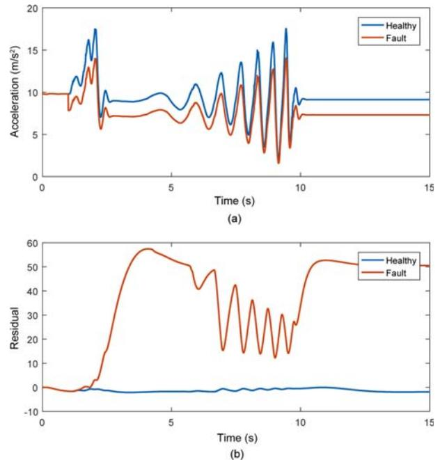
Figure 11. Wavy uphill road simulation results for residual generation (gain fault): (a) Front left sprung mass acceleration; (b) Residual generated by the unknown input residual generator.
