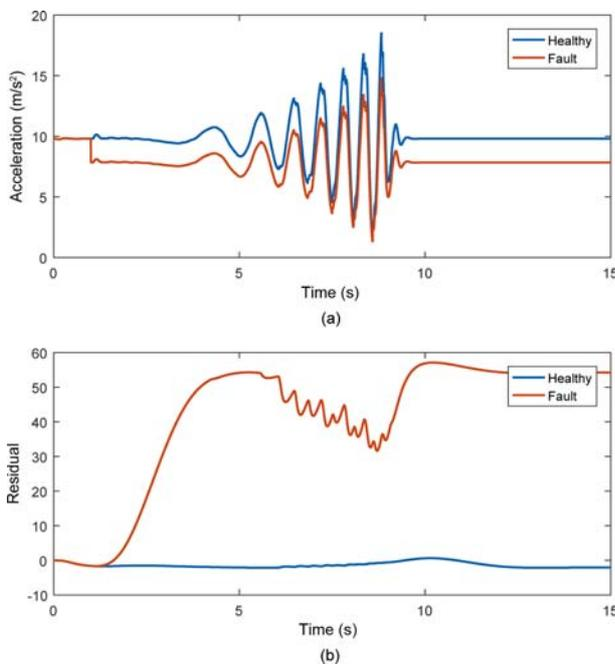
Figure 5. Wavy road simulation results for residual generation (gain fault): (a) Front left sprung mass acceleration; (b) Residual generated by the unknown input residual generator.
