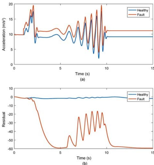
Figure 12. Wavy uphill road simulation results for residual generation (bias fault): (a) Front left sprung mass acceleration; (b) Residual generated by the unknown input residual generator.
