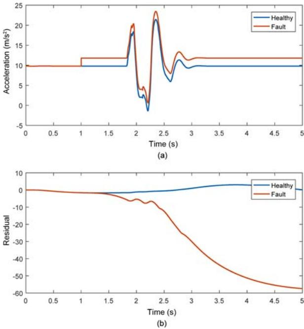
Figure 9. Speed-bump simulation results for residual generation (bias fault): (a) Front left sprung mass acceleration; (b) Residual generated by the unknown input residual generator.
