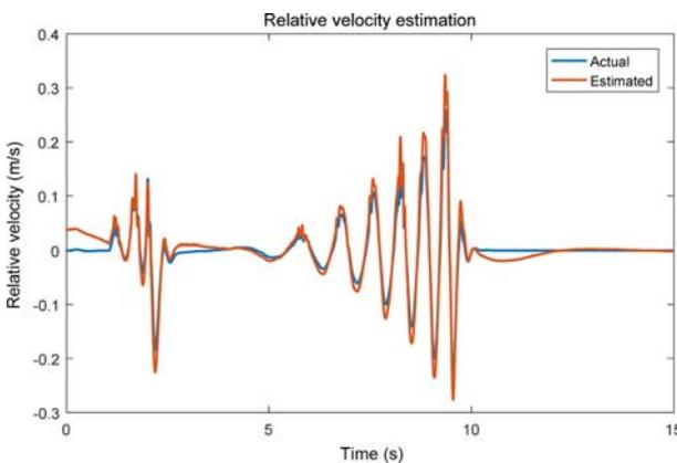
Figure 13. Wavy uphill road simulation results for the relative velocity estimation: Front left suspension relative velocity.
