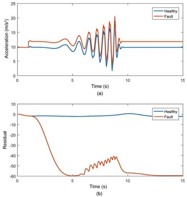
Figure 6. Wavy road simulation results for residual generation (bias fault): (a) Front left sprung mass acceleration; (b) Residual generated by the unknown input residual generator.
