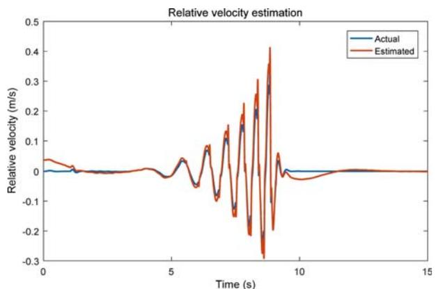
Figure 7. Wavy road simulation results for the relative velocity estimation: Front left suspension relative velocity.
