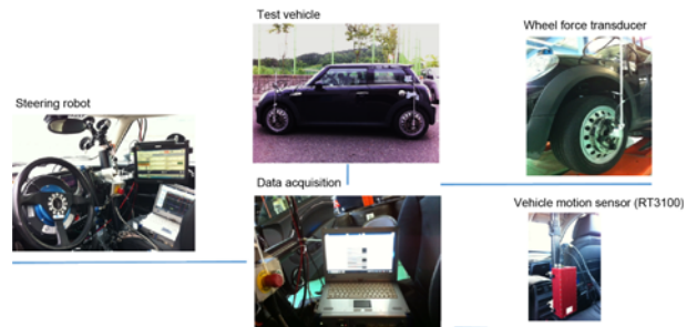
Figure 3. Implementation of data acquisition devices for the estimator validation.
