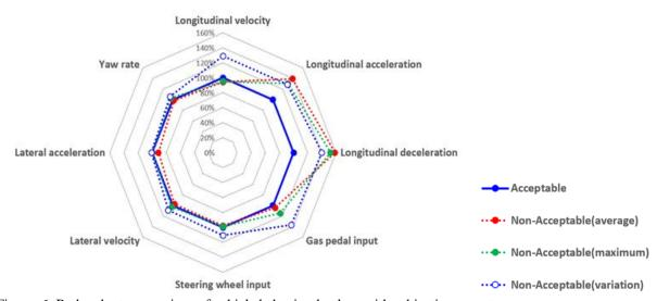
Figure. 6: Radar chart comparison of vehicle behavioral values with subjective acceptance
