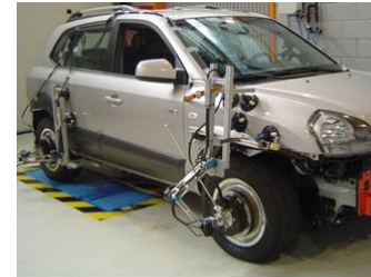
Figure 7. Test vehicle : full size SUV equipped with wheel force transducer
