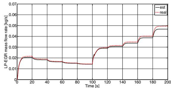
Figure 8 shows the difference of LP-EGR mass flow rate depending on operating points. Precise estimation of LP-EGR mass flow rate is difficult because it was assumed that temperature sensor is not equipped in LP-EGR pipe. Uncertainty of LP-EGR pipe is connected to model uncertainty. Model uncertainty can affect asymptotical stability of the observer. In figure 7, slight offset appeared due to inaccuracy of LP-EGR mass flow rate.
