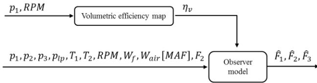
Figure 2 shows the prerequisites of suggested burnt gas fraction estimation. It was assumed that pressure, temperature and MAF data is obtained through sensors. Volumetric efficiency map was designed by experiment as a function of intake manifold pressure and RPM.
