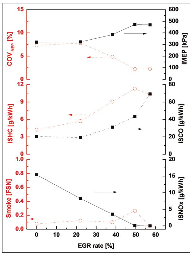
**Figure 5.** IMEP, COV of IMEP and emissions at injection timing of 40°CA BTDC with the EGR rate for the baseline injector (8H146). Engine speed, injection pressure and injection quantity were 1200 r/min, 160 MPa and 30 mg/stroke, respectively.
