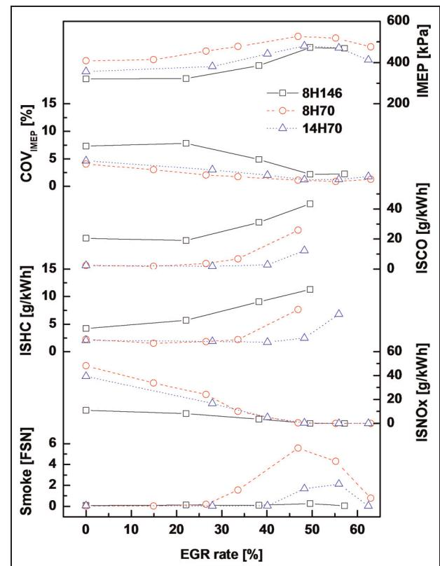
**Figure 7.** IMEP, COV of IMEP and emissions at injection timing of  $40^\circ$ CA BTDC according to the EGR rate for various injectors. Engine speed, injection pressure and injection quantity were 1200 r/min, 160 MPa and 30 mg/stroke, respectively.
