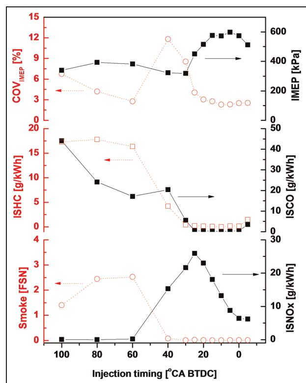
**Figure 3.** IMEP, COV of IMEP and emissions according to the injection timing for baseline injector (8H146). Engine speed, injection pressure and injection quantity were 1200 r/min, 160 MPa and 30 mg/stroke, respectively.
