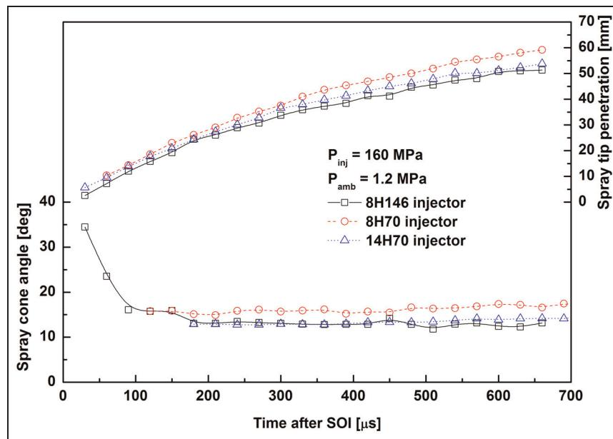
**Figure 9.** Spray tip penetration and spray cone angle versus time after the start of injection with respect to the injector configurations.
