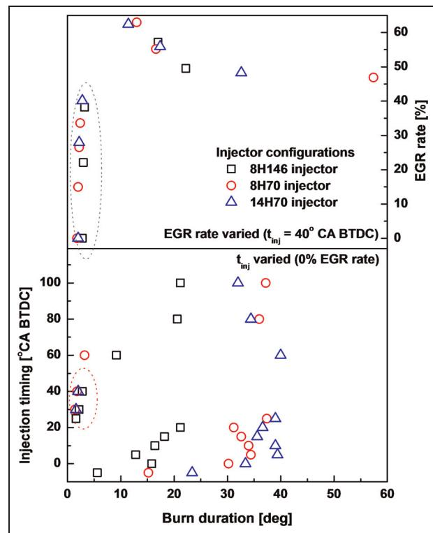
**Figure 6.** Burn duration for the various injector configurations with respect to EGR rate at a fixed injection timing of  $40^\circ$ CA BTDC (top) and to the injection timing at EGR rate of 0% (bottom). Engine speed, injection pressure and injection quantity were 1200 r/min, 160 MPa and 30 mg/stroke, respectively.
