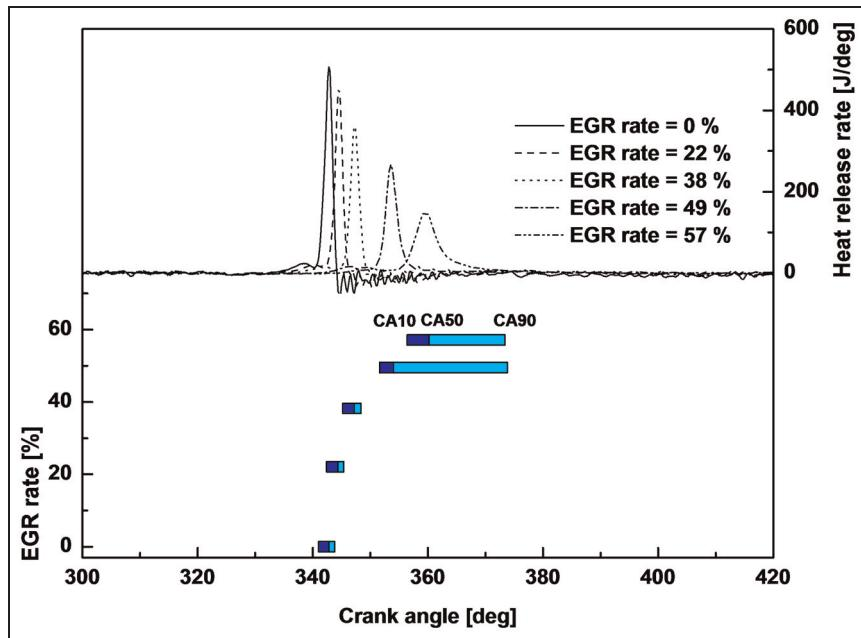
**Figure 4.** Heat release rate and burn duration with the EGR rate at injection timing of 40°CA BTDC for baseline injector (8H146). Engine speed, injection pressure and injection quantity were 1200 r/min, 160 MPa and 30 mg/stroke, respectively.
