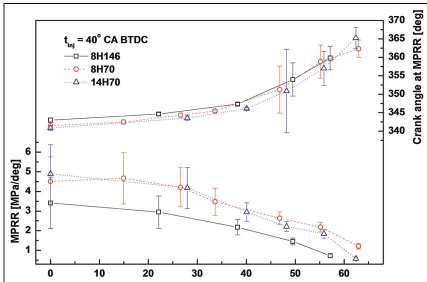
**Figure 10.** The maximum pressure rise rate (MPRR) and crank angle corresponding to the MPRR according to the EGR rate for three injector configurations at injection timing of 40°CA BTDC. Engine speed, injection pressure and injection quantity were 1200 r/min, 160 MPa and 30 mg/stroke, respectively.
