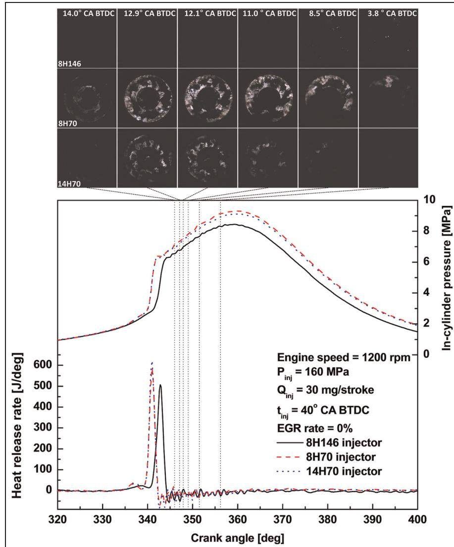
**Figure 8.** In-cylinder visualization, pressure and heat release rate in terms of the injector configurations at injection timing of 40°CA BTDC and without EGR. Engine speed, injection pressure and injection quantity were 1200 r/min, 160 MPa and 30 mg/stroke, respectively.
