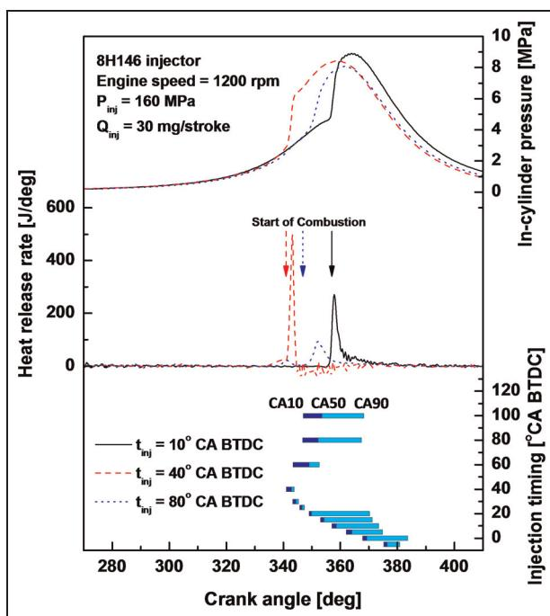
**Figure 2.** In-cylinder pressure, heat release rate and burn duration according to the injection timing including the injection timing of  $10^{\circ}$ ,  $40^{\circ}$  and  $80^{\circ}$ CA BTDC for baseline injector (8H146). Engine speed, injection pressure and injection quantity was 1200 r/min, 160 MPa and 30 mg/stroke, respectively.
