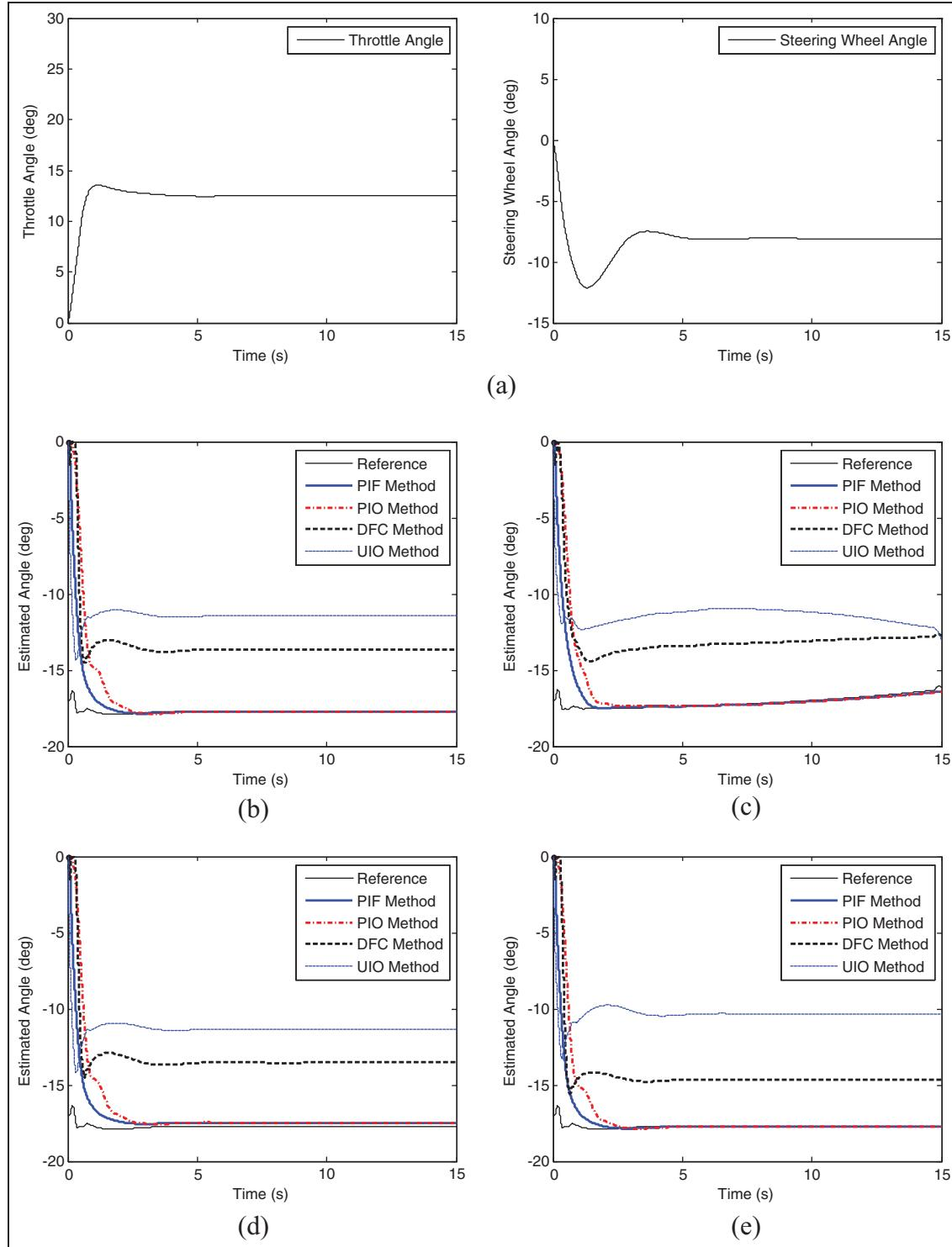
**Figure 2.** Simulation results (constant road bank angle): (a) driver inputs; (b) estimated  $\varphi$  ( $\mu = 0.85$ ); (c) estimated  $\varphi$  ( $\mu = 0.3$ ); (d) estimated  $\varphi$  ( $a_y = a_{y\_real} \cos(10^\circ)$ ); (e) estimated  $\varphi$  ( $C_f = 1.2C_{f\_ss}$ ).
