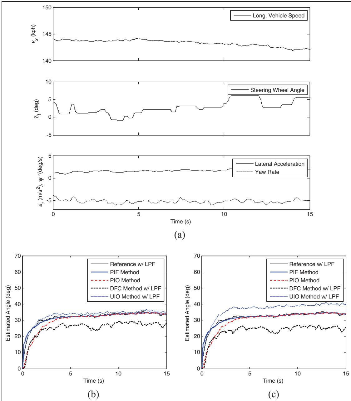
**Figure 6.** Test results (lane 1): (a) vehicle states from sensors; (b) estimated  $\varphi$  ( $C_f = C_{f\_ss}$ ); (c) estimated  $\varphi$  ( $C_f = 1.2C_{f\_ss}$ ). Long.: longitudinal; w/ LPF: with a low-pass filter; PIF: proportional–integral  $H_\infty$  filter; PIO: proportional–integral observer; DFC: dynamic filter compensation; UIO: unknown input observer.
