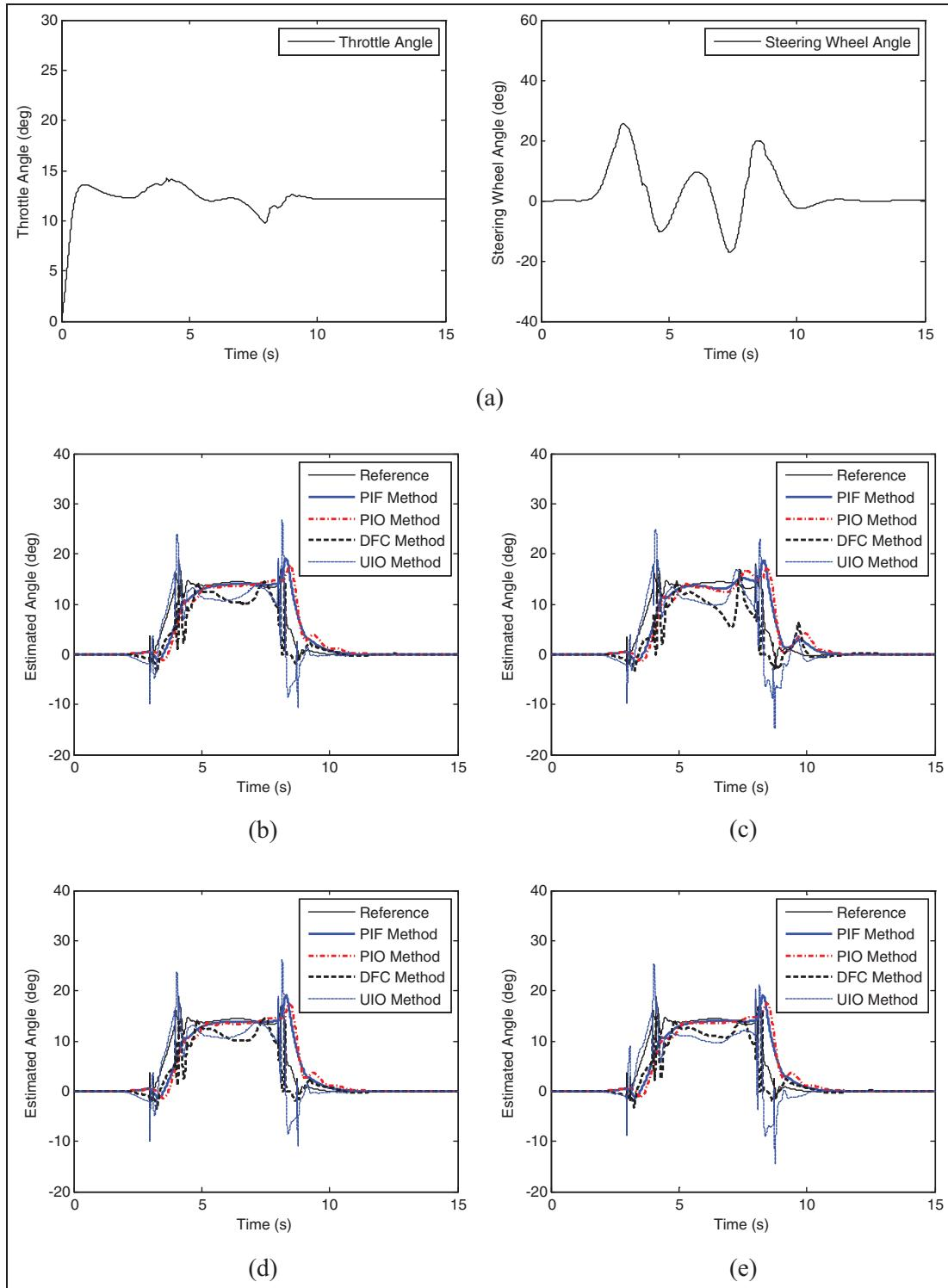
**Figure 3.** Simulation results (double lane change on a flat road): (a) driver inputs; (b) estimated  $\varphi$  ( $\mu = 0.85$ ); (c) estimated  $\varphi$  ( $\mu = 0.3$ ); (d) estimated  $\varphi$  ( $a_y = a_{y\_real} \cos(10^\circ)$ ); (e) estimated  $\varphi$  ( $C_f = 1.2C_{f\_ss}$ ).
