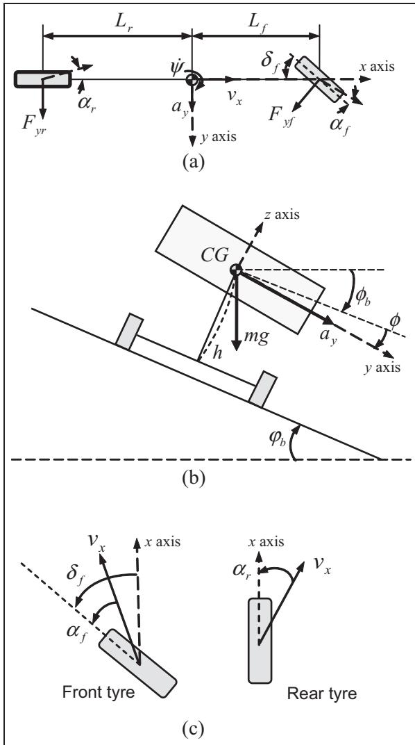
**Figure 1.** Schematic diagrams of the target system: (a) bicycle model of a vehicle; (b) rear view of a vehicle; (c) tyre diagram. CG: centre of gravity.
