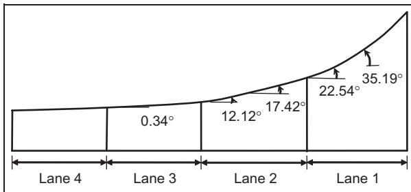
**Figure 5.** Test lanes and road bank angle status.
