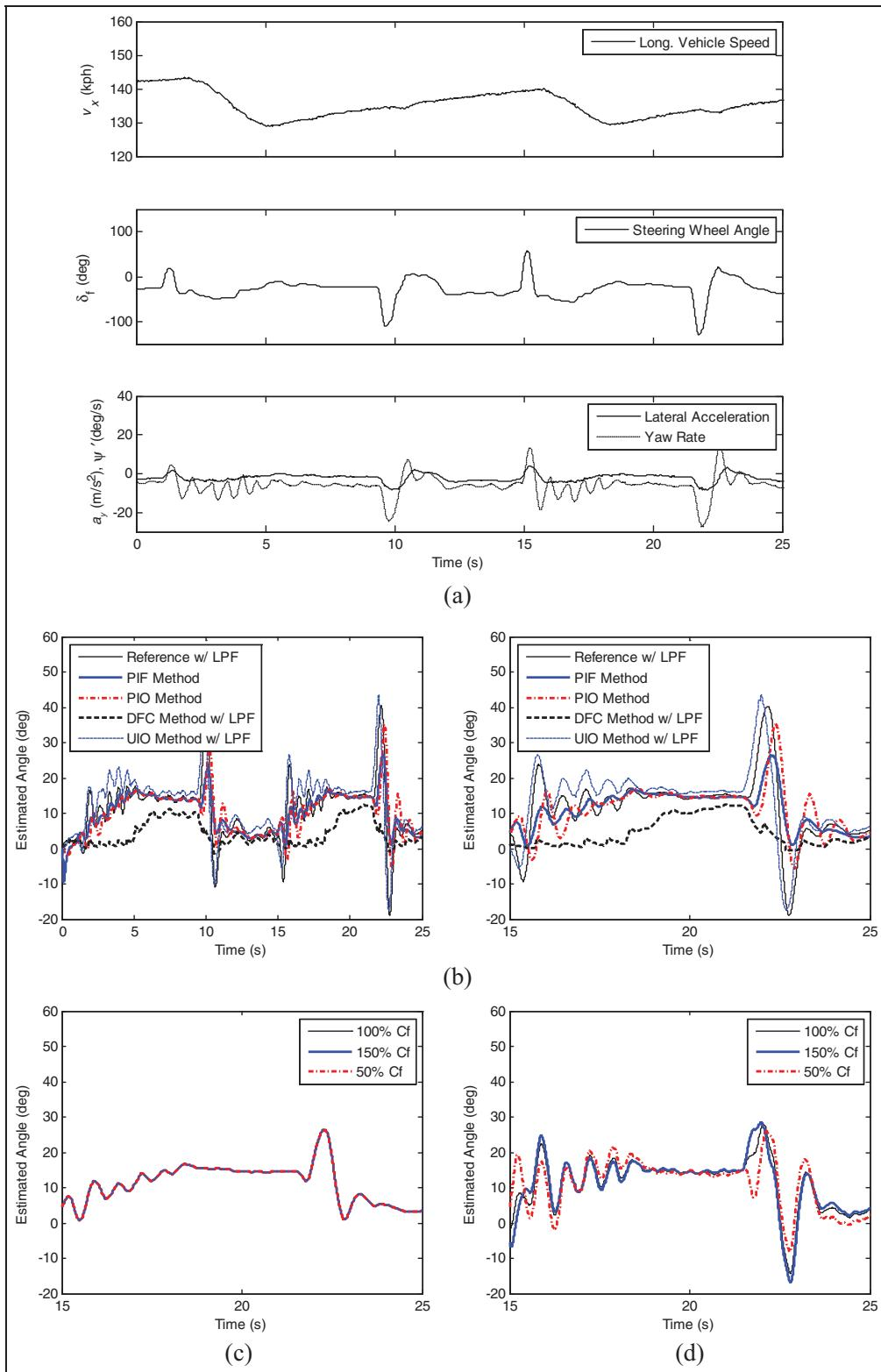
**Figure 7.** Test results (lane 2  $\leftrightarrow$  lane 3): (a) vehicle states from sensors; (b) estimated  $\varphi$ ; (c) robustness of PIF with the modified vehicle model; (d) robustness of PIF with the original vehicle model.
