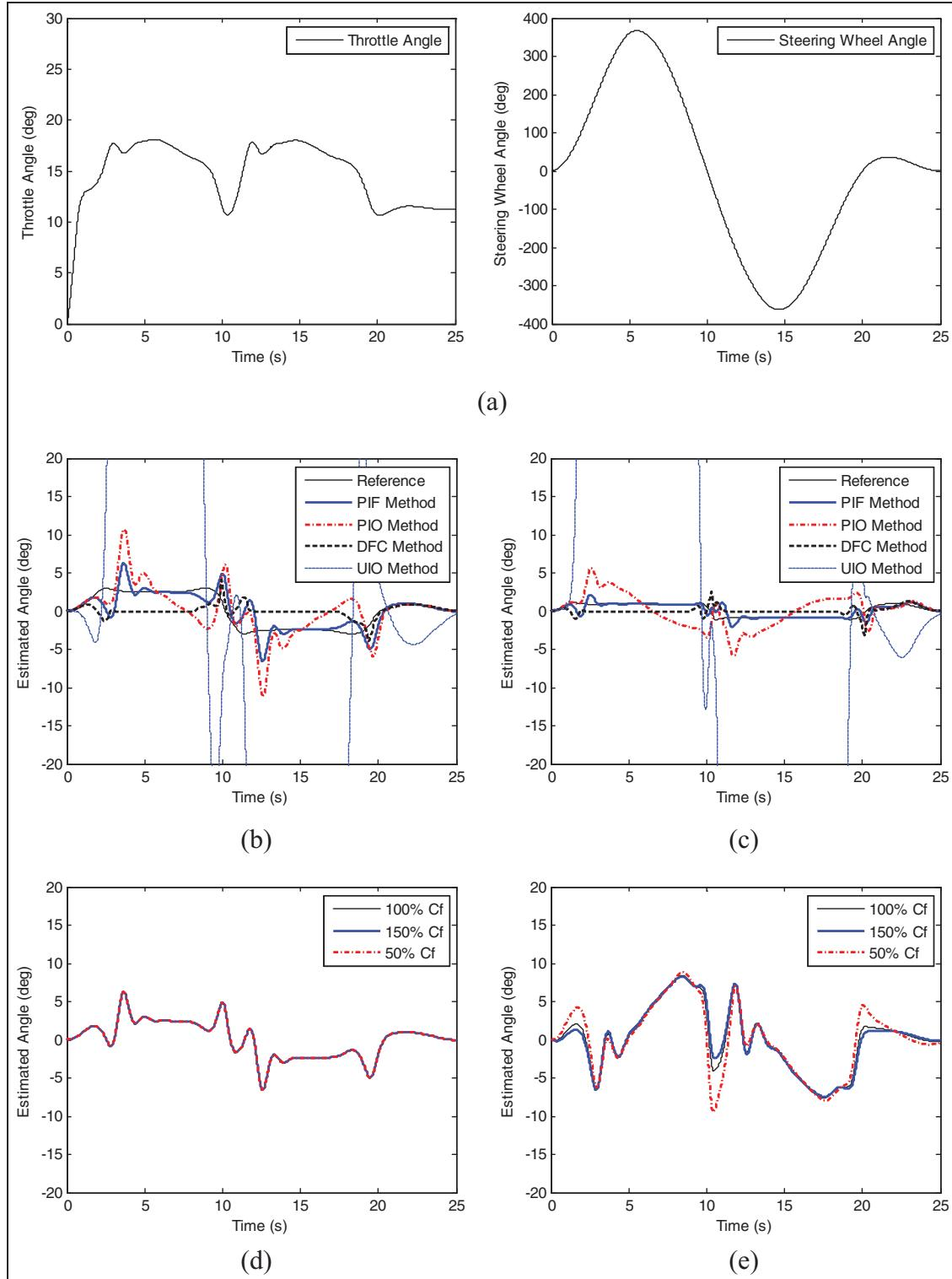
**Figure 4.** Simulation results (S-curve manoeuvre on a flat road): (a) driver inputs; (b) estimated  $\varphi$  ( $\mu = 0.85$ ); (c) estimated  $\varphi$  ( $\mu = 0.3$ ); (d) robustness of PIF with the modified vehicle model ( $\mu = 0.85$ ); (e) robustness of PIF with the original vehicle model ( $\mu = 0.85$ ).
