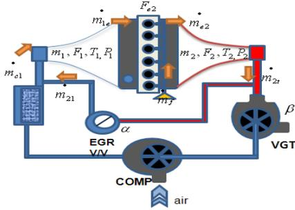
Figure 1-Diesel engine model
