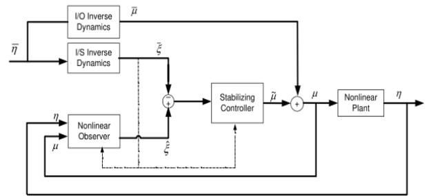
Figure 4. Trajectory linearization scheme
