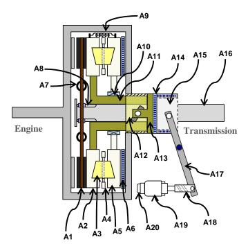
Figure 3: Clutch actuator mechanism
