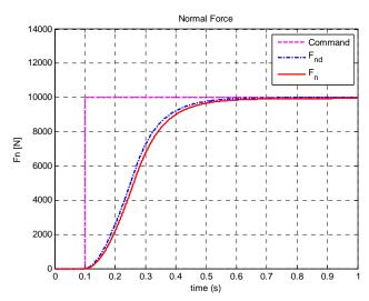
Figure 6: Simulation result: feedback control (alpha=28 deg)
