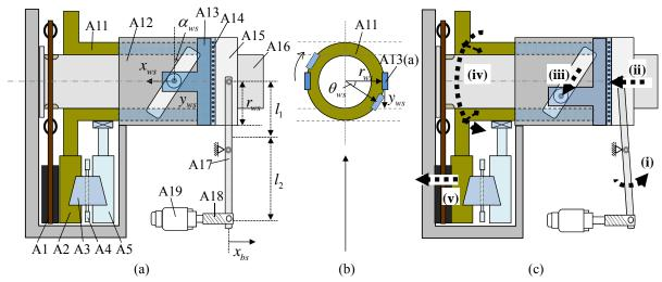
Figure 4: Operation principle of the clutch actuator system (a) Disengaged phase. (b) Cross section of the worm shaft. (c) Engaged phase.
