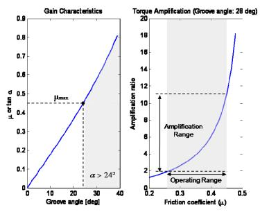
Figure 5: Torque amplification characteristics
