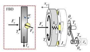
Figure 2: Schematic of the new clutch actuator system
