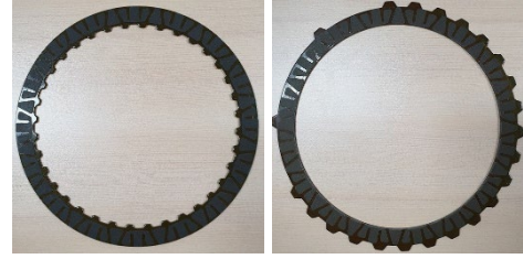
Figure 8. Single-sided clutches. Outer-toothed clutch disk (left). Inner-toothed clutch disk (right)
