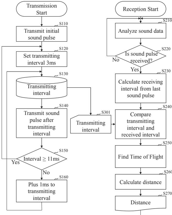
Fig. 4. Flow chart of the proposed ultrasonic distance sensing algorithm.
