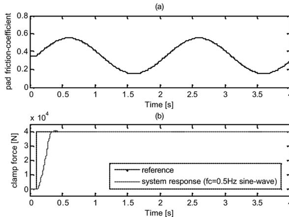
The simulation result in Figure 9 shows that the proposed controller is robust even if the pad friction-coefficient varies during a single braking.
