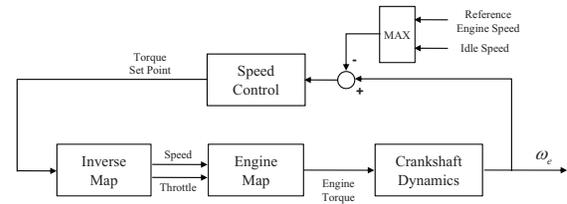
Fig. 6. Block diagram of the engine speed/torque control
