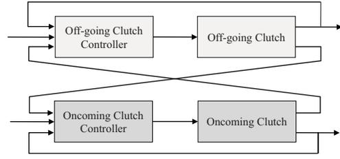
Fig. 5. Schematic of the control concept for DCTs
