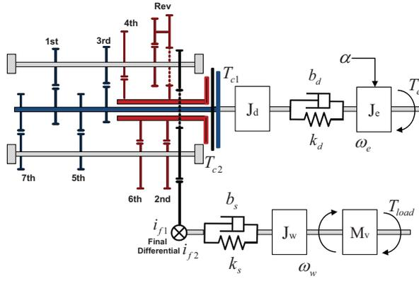
Fig. 1. Vehicle driveline dynamics with a DCT
