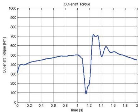
Fig. 9. Output shaft torque in 1-2 upshift
