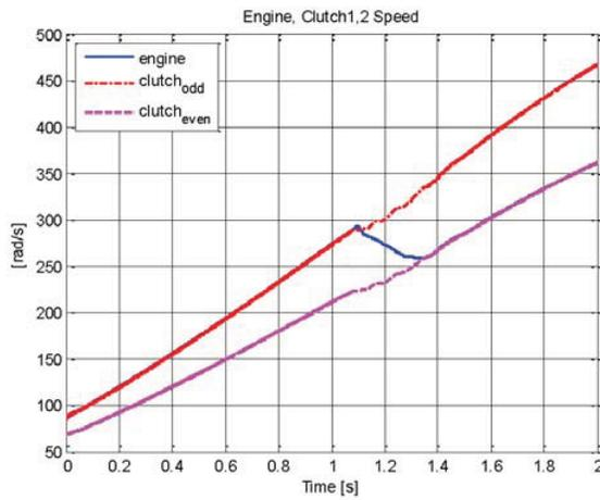
Fig. 7. Engine and clutch speeds during 1-2 upshift
