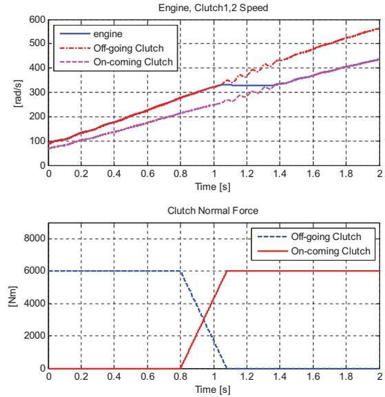
Fig. 4. Open-loop based control for gear shifting (1-2 upshift)
