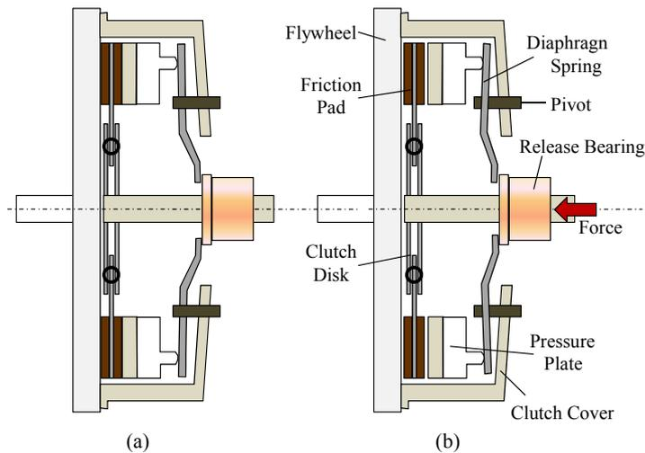
Figure 1: Conventional clutch actuator system for manual transmissions
