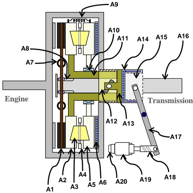
Figure 3: Clutch actuator mechanism
