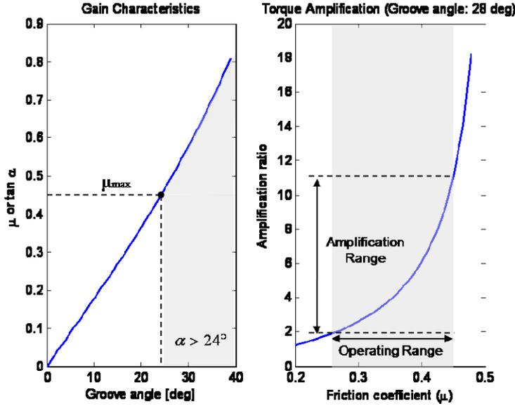
Figure 5: Torque amplification characteristics
