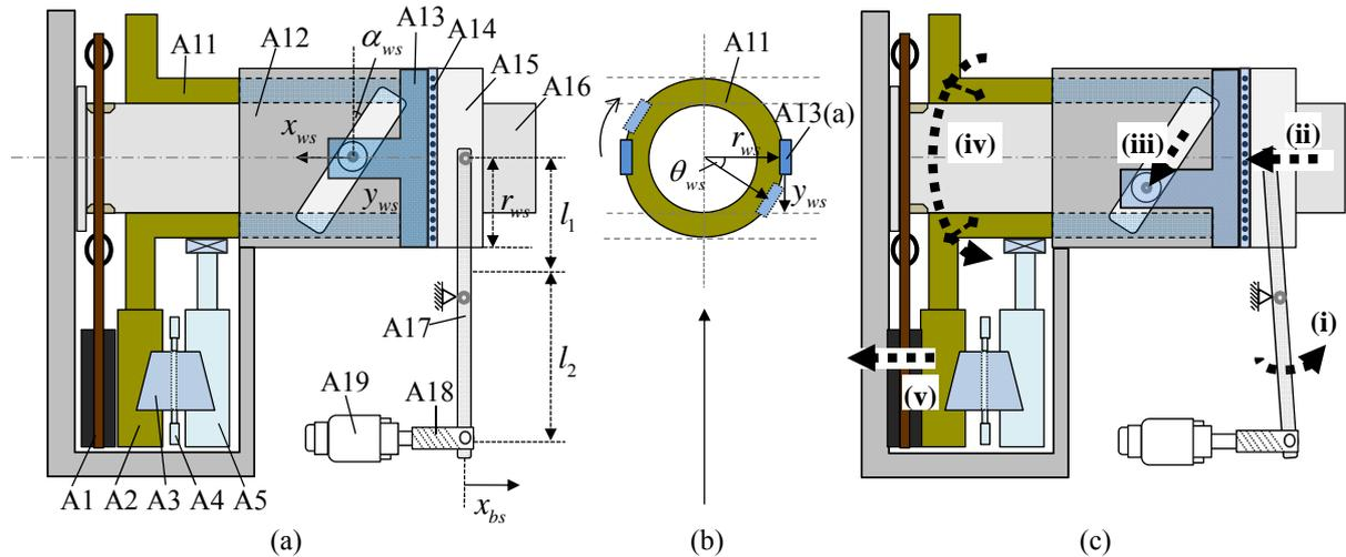
Figure 4: Operation principle of the clutch actuator system (a) Disengaged phase. (b) Cross section of the worm shaft. (c) Engaged phase.
