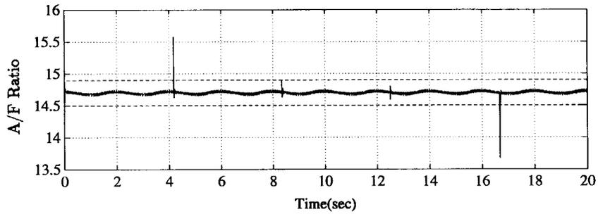
Fig. 9. A/F ratio by dynamic sliding mode control without measurement time delay (simulation).
