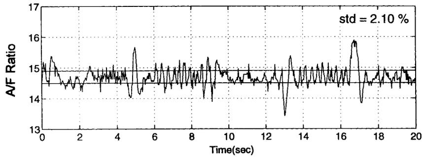
Fig. 13. A/F ratio controlled by production ECM.
