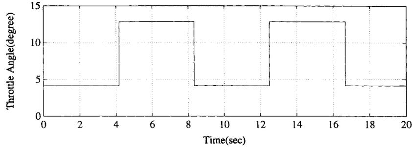
Fig. 8. Throttle angle pattern in A/F ratio control simulation.
