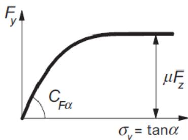
Fig. 1 Lateral tire force versus wheel side slip angle (5) has always positive solution because  $C_\alpha |\tan(\alpha)| - F_y$  is always semi-positive.
