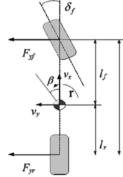
Fig. 3 Bicycle model for vehicle lateral dynamics.
