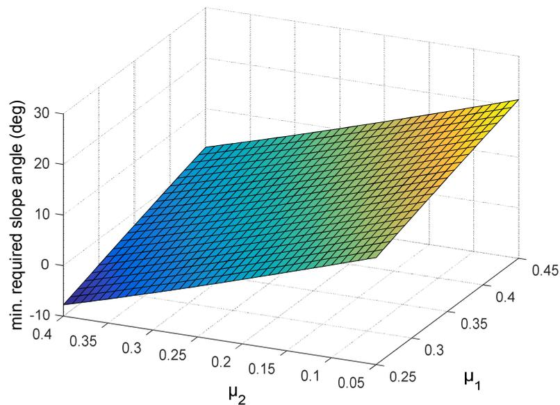
Figure 6. Minimum slope angle for locking avoidance.
