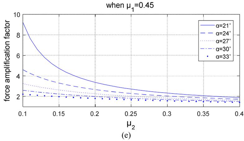
Figure 5. Variations in the force amplification factor according to  $\mu_2$  and  $\alpha$  for (a)  $\mu_1 = 0.25$ , (b)  $\mu_1 = 0.3$ , (c)  $\mu_1 = 0.35$ , (d)  $\mu_1 = 0.4$ , and (e)  $\mu_1 = 0.45$ .
