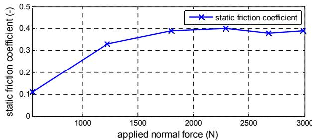
Figure 4. Static friction coefficient characteristics of the clutch.
