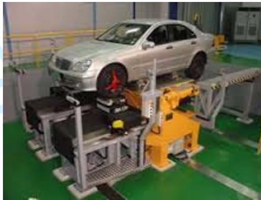
Figure 7 Suspension parameter test machine [11]
