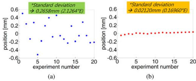
Fig. 10. Experimental verification of the initial position aligning method: (a) aligned by eye and (b) aligned by  $V_\alpha$  application.
