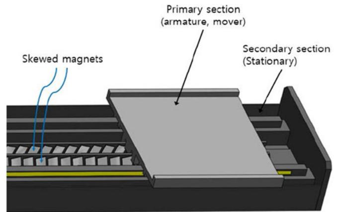
Fig. 6. Skewed permanent magnets.
