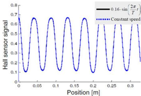
Fig. 2. Hall sensor signal at identical position with different travel speeds. (Black solid line: sinusoidal position trajectory with period  $T$  of 1, 2, 4, 6, and 8 s, and 0.32 m stroke, blue dotted line: constant speed of 0.02, 0.06, 0.10, 0.15, and 0.20 m/s.)
