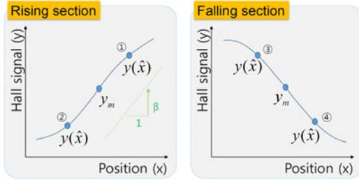
Fig. 7. Sensor signal model decomposition into two sections.
