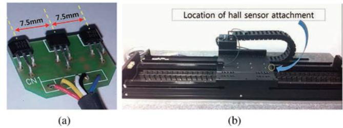
Fig. 1. Hall sensor array on (a) PCB and (b) applied linear motor system.
