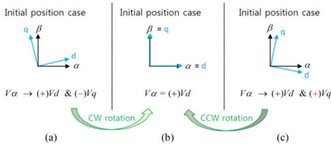
Fig. 9. Initial position aligning mechanism by applying  $V_\alpha$ .
