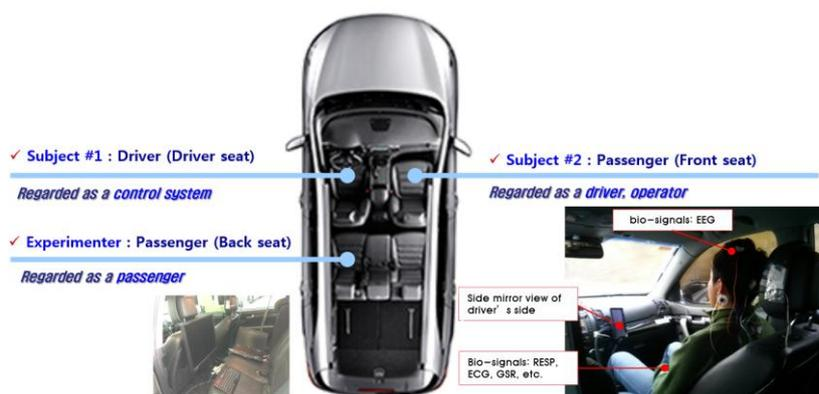
Figure 1: Configuration of test environments for passengers
