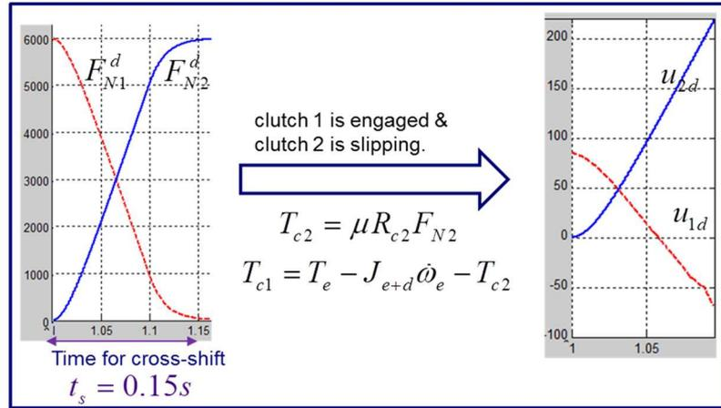
Figure 3: Design of  $u_d$  for control allocation
