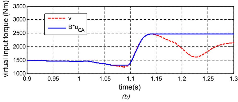
Figure 5: Control allocation results when  $W_u = I$ ,  $W_v = 10$
