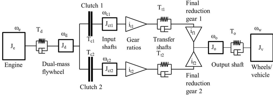
Figure 2: Schematic of the DCT driveline model
