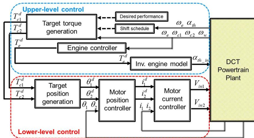
Figure 1: General structure of dry DCT powertrain controls
