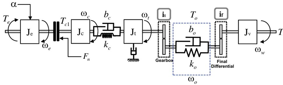
Fig. 1. Vehicle driveline diagram
