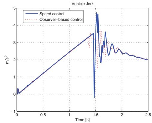
Fig. 9. Simulation results for vehicle jerk: speed control and observer-based torsion control for clutch engagement during a vehicle launch
