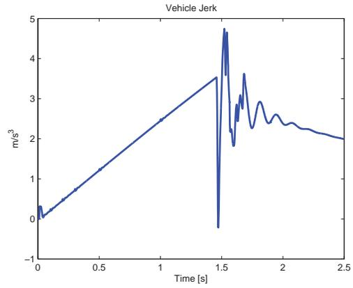
Fig. 5. Modified speed control for clutch engagement during a vehicle launch: vehicle jerk
