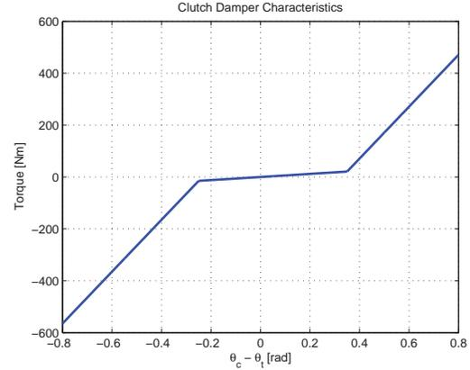
Fig. 2. Clutch damper characteristics
