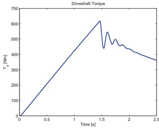
Fig. 4. Modified speed control for clutch engagement during a vehicle launch: Output torque
