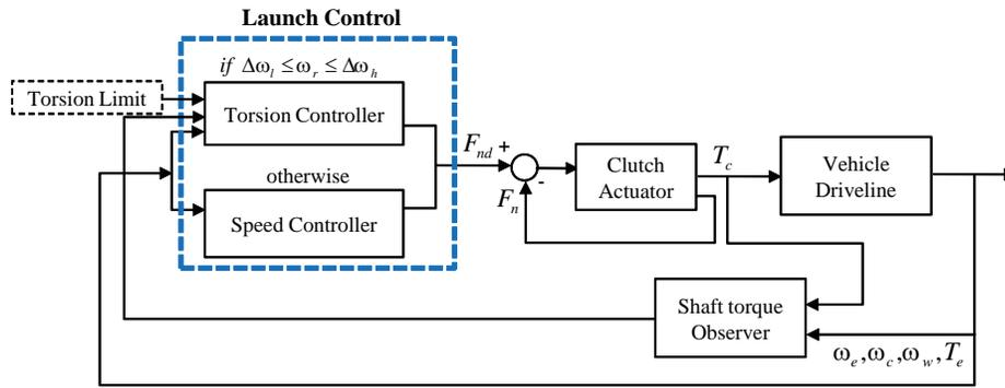
Fig. 10. Structure of the speed-torsion controller with shaft torque observer
