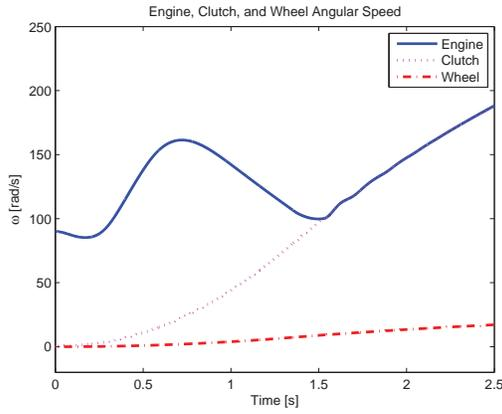
Fig. 6. Torsion control for clutch engagement during a vehicle launch: Angular speed of each element
