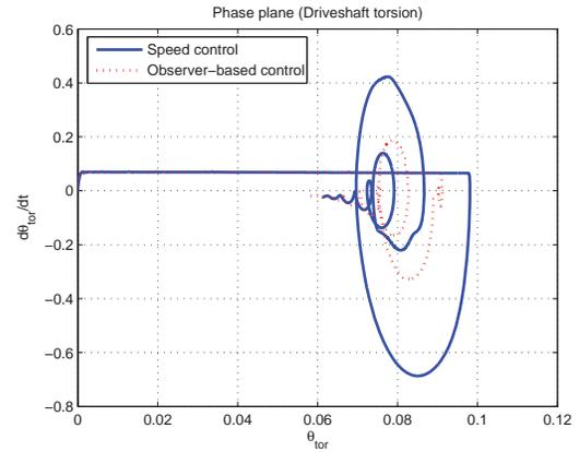
Fig. 8. Simulation results for the phase plane of shaft torsion: speed control and observer-based torsion control for clutch engagement during a vehicle launch
