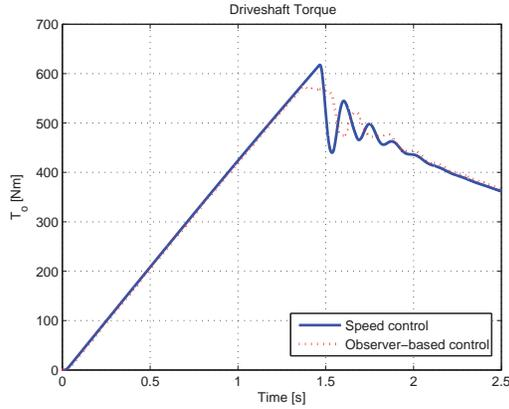
Fig. 7. Simulation results for the output torque: speed control and observer-based torsion control for clutch engagement during a vehicle launch
