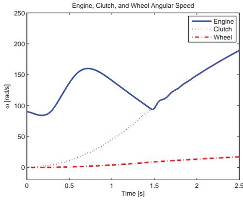
Fig. 3. Modified speed control for clutch engagement during a vehicle launch: angular speed of each element
